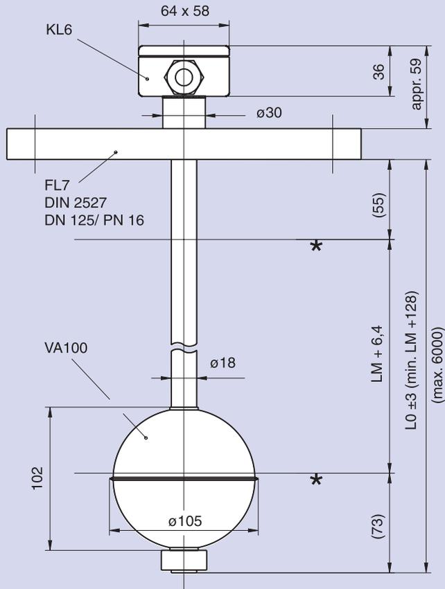
★ Immersion depth at density 1: VA100 = 52 ± 3 mm, BN42 = 33 ± 2 mm
