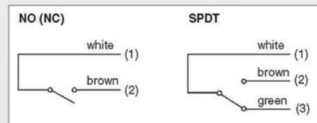
By turning the float upside down the function of the switch contact can be changed from NO (standard) in NC or vice versa. (Not possible with SPDT contacts).
