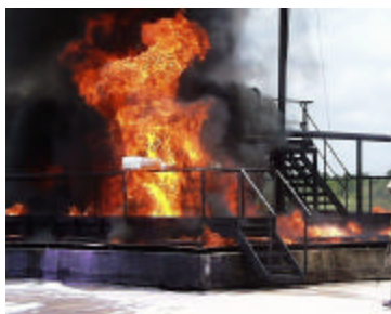
Hydrocarbon Pool Fire
