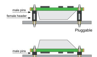
Soldered single pin header
