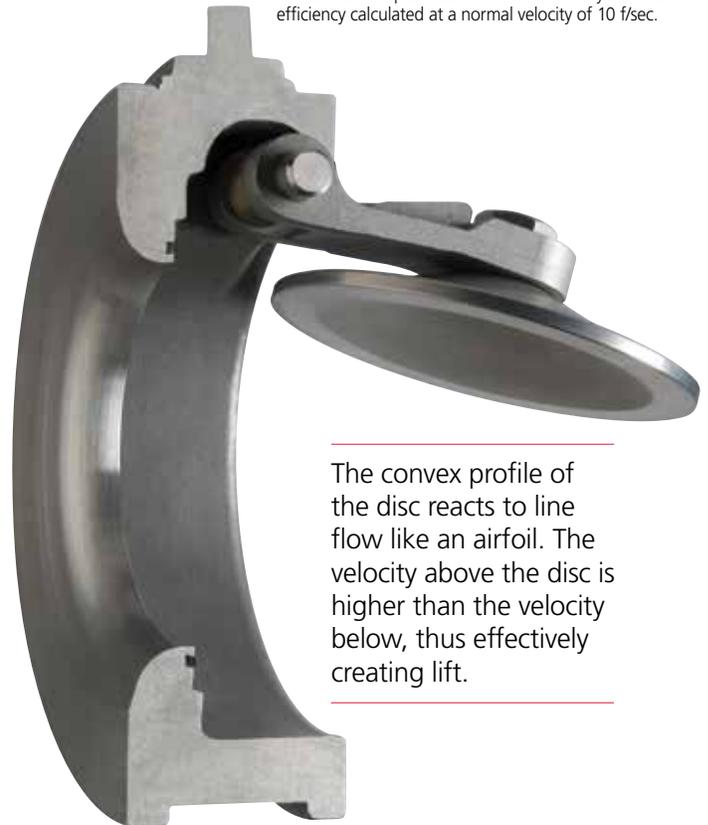
The convex profile of the disc reacts to line flow like an airfoil. The velocity above the disc is higher than the velocity below, thus effectively creating lift.
