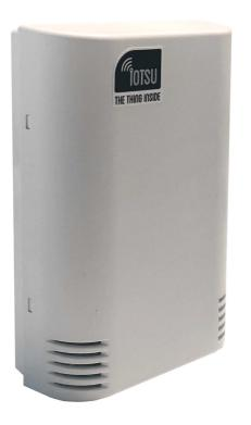
IOTSU® TH02 is a compact wireless indoor device that measures air temperature and relative humidity. IOTSU® is a perfect solution for long-time monitoring of temperature and humidity of real estates and building structures.
