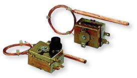
LS1 / LS3 is a capillary thermostat with a liquid expansion probe, unipolar, with safety temperature limiter with manual or automatic reset and with positive safety in case of capillary breakage. It is particularly suitable for boilers, heating systems and in all those appliances where it is necessary not to exceed a maximum set temperature.
