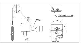
Switches = interrupted due to temperature increase Max. head temperature = 85°C Copper bulb = 125°C Copper bulb = Ø 6,5 x 95 mm Min. capillary curvature radius = 5 mm Certifications = CE, ENECO3, EAC, UL, CSA
