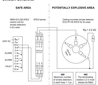
The alarm and fault relay contacts are displayed in de-energised/ alarm condition. Alarm relay max 8A, 250V. Fault relay max 5A, 250V.
