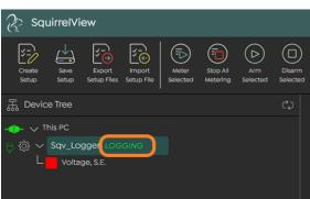
When the Delayed Start timer conditions are met LOGGING will be displayed, informing you that the logger is recording data.
