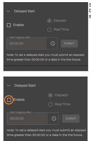
Scroll to the bottom of the tab's window, until the Delayed Start settings are displayed. (by default these will be disabled)
