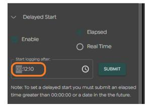
The time delay can also be directly entered by clicking on the 'start logging after' time and typing valid values.
