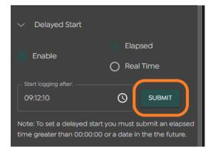
Press the Submit button to send the elapsed timer settings to the logger.
