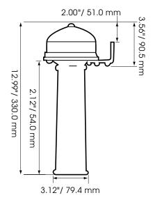
Model VS-111EMS is an electrical/mechanical buzzer ideal for applications requiring a low frequency and penetrating audible signal. VS-111EMS is a single stage alarm that produces a unique tone caused by a vibrating diaphragm. They can also be pulsed by a control panel/PLC to produce an intermittent signal.
