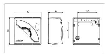
Electrical contact capacity = 16(2,5) A / 250 Vac Regulation range = 5°÷30°C
