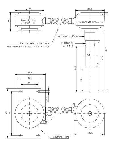
> remote electronics installation with angled screw coupling
