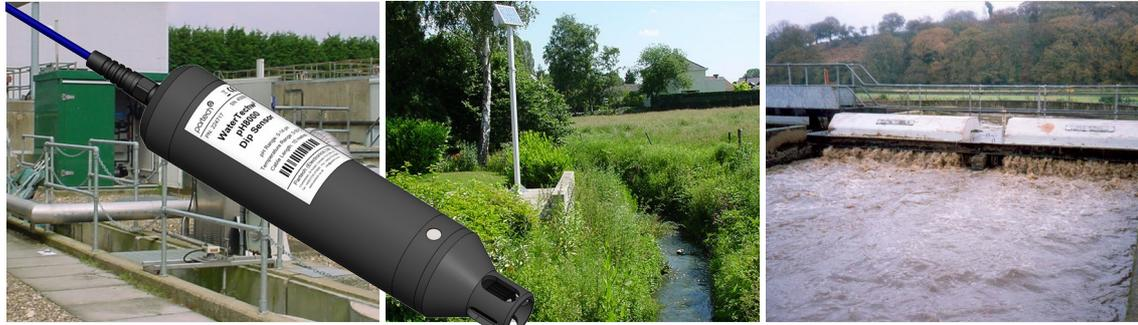
Measurement of Redox or ORP is useful in many water, wastewater and industrial water processes, for example the control of disinfection processes such as chlorination in cooling towers. The electrode design is very similar to the equivalent pH electrode (WaterTechw<sup>2</sup> pH8000), the difference being that the pH glass is replaced with a Platinum band.
