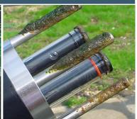
The TurbiTechw<sup>2</sup> LS Sensor is designed to monitor the levels of Suspended Solids or Turbidity typically found in Final Effluent from municipal and industrial wastewater treatment plants. It is also capable of monitoring solids in the intake to both effluent and drinking water treatment processes. The normal operating range is between 0 - 500 FTU, with versions of the sensor suitable for 0-100FTU and 0-1,000 FTU ranges available.
