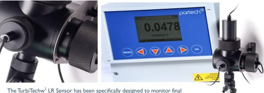
treated, portable and filter water. The sensor is extremely sensitive and is capable of discriminating changes in Turbidity of less than 0.1 FTU. The 90° light scatter monitoring technique makes the sensor sensitive to a wide range of particle sizes, from colloidal material through to larger particles and raw waters and the large mineral particles sometimes found in distribution samples.
