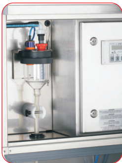
Pneumatic dosing system with capacitive Ex-sensor
