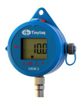
The TV-4804 measures current from 0 to 25mA DC and can be connected to a variety of industry standard sensors enabling the logging of a wide range of process parameters.
