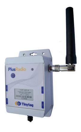
Tinytag Plus Radio data loggers are a range of wireless data logging products designed for outdoor and industrial use. The loggers are used as part of a Tinytag Radio system that forms a robust data network that allows a user to see the conditions within an application from their own desk, across a LAN or the Internet.
