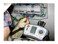
The instrument features a test button in the probe and a lockdown test button for 'hands free' operation.
