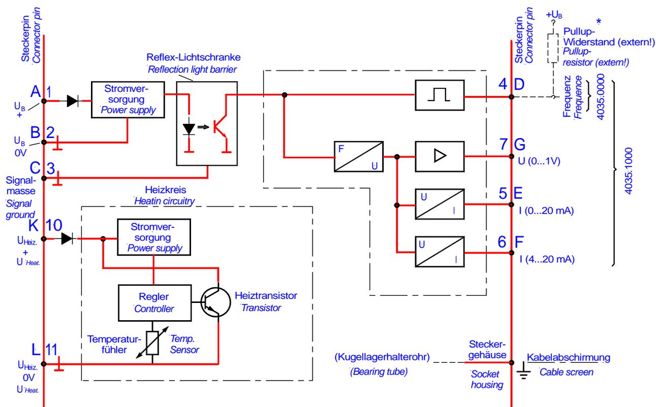
**Attention:** When several analog outputs are used simultaneously, each output requires a separate ground wire to be installed directly close to the sensor.
