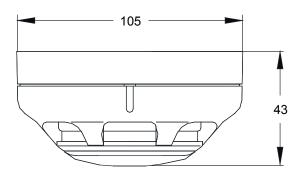
Mounting: 2 x M4 screws, 50 / 60 / 70 mm c/c
