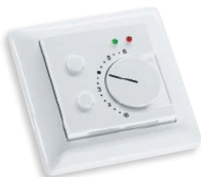
FSTF xx P2L2T Version with sensor, potentiometer (1 kOhm, max. 0.1 W), 2 LEDs (green, red), and 2 push-buttons (max. 24 V DC, max. 10 mA)
