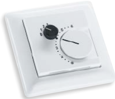
FSTFxxPD4 Version with sensor, potentiometer (1 kOhm, max. 0.1 W) and turn switch (max. 24 V AC / DC, max. 130 mA)
