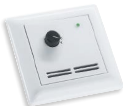
FSTF xx LD2 Version with sensor, LED (green), and turn switch (2-step) (max. 24 V AC / DC, max. 130 mA)
