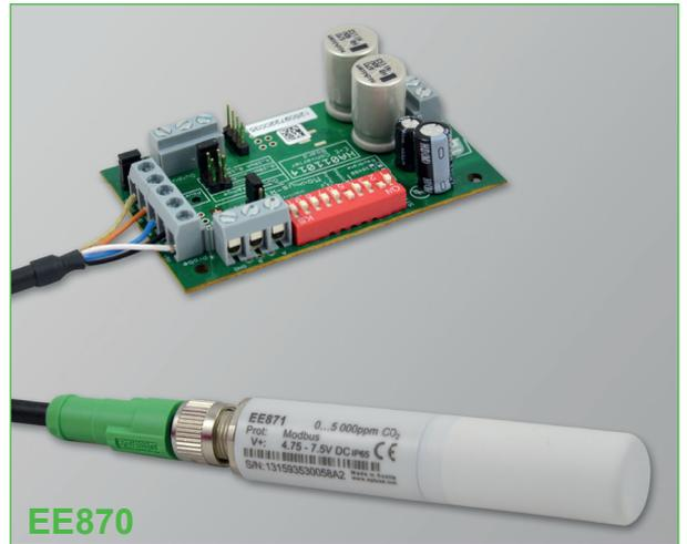
The measured data range of up to 5 % CO<sub>2</sub> (50,000 ppm) is available on the analog outputs of the conversion board. Several voltage and current ranges can be selected with jumpers. Additionally, the data is available on the Modbus RTU interface, which can be configured by the user with DIP switches on the board. An optional kit facilitates easy configuration and adjustment of the probe.
